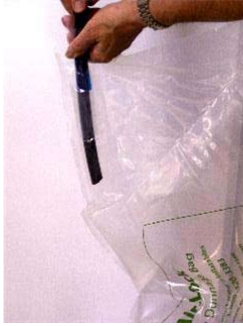
Step 3. While holding valve in left hand, push deflator completely into valve.
