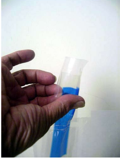
Step 1. Open valve with blue side facing you, by rolling between thumb and index finger.
